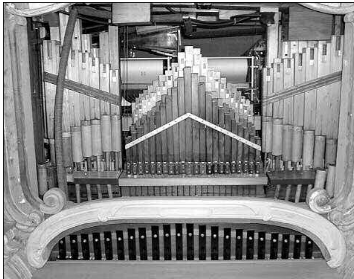
Figure 1. The mid-section of the Wurlitzer 165 military band organ, serial # 2992. Note the myriad of pipes along with the bells below and the twin roll frames in the background.
